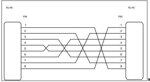
Figure 17: Crossed RJ-45 Cable BayTech Part No. RJ08X010 (10 feet)
